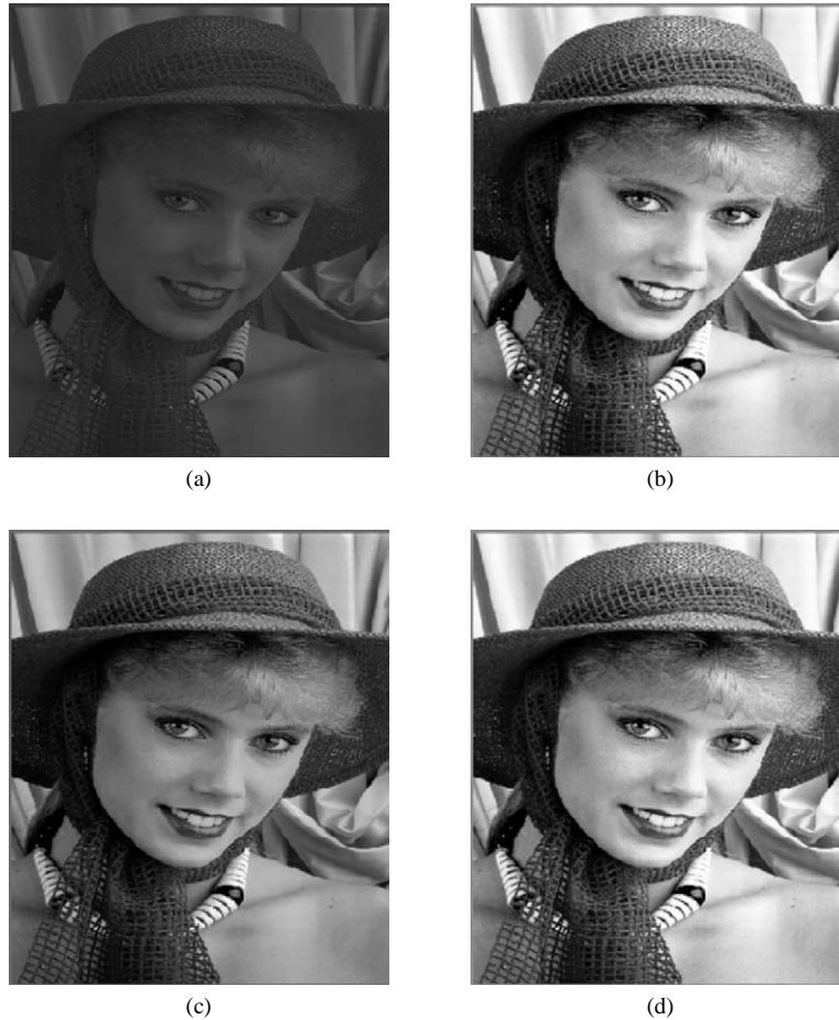
Fig. 4. The comparison of enhancement using different approaches for a dark image. (a) Original image, (b) HE, (c) multi-peak HE, (d) multi-peak GHE ( \alpha = 50 , \beta = 0.01 ), (e) original image, (f) HE, (g) multi-peak HE, and (h) multi-peak GHE.
