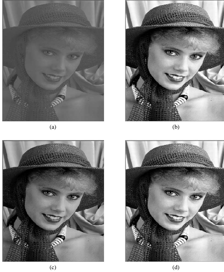
Fig. 3. The comparison of enhancement using different approaches. (a) Original image, (b) HE, (c) multi-peak HE, (d) multi-peak GHE ( \alpha = 50 , \beta = 0.01 ), (e) original image, (f) HE, (g) multi-peak HE, and (h) multi-peak GHE.
