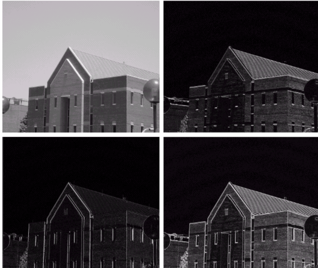
FIGURE 10.10 (a) Original image. (b) |G_x| , component of the gradient in the x -direction. (c) |G_y| , component in the y -direction. (d) Gradient image, |G_x| + |G_y| .
