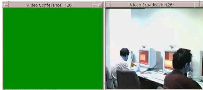
Figure 11: AES: encrypt only 16-bytes using H261 encoder
