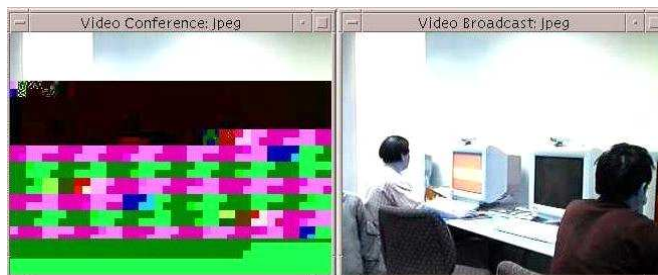
Figure 9: AES: encrypt only 128-bytes using JPEG encoder
