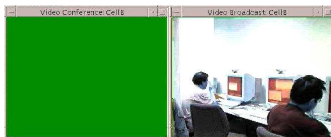
Figure 12: AES: encrypt only 16-bytes using CellB encoder
